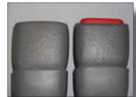
A comparison of the Gen 2 and Gen 3 seat belt buttons. The Gen 3 had a button that protruded from the cover.
